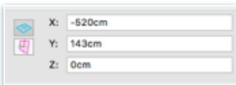
In the first example (base). when the "Z" of the parametric object is set to 0, also the point indicated as origin will be placed at Z=0.
